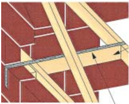
Figure 102 Restraint strap at ceiling level
