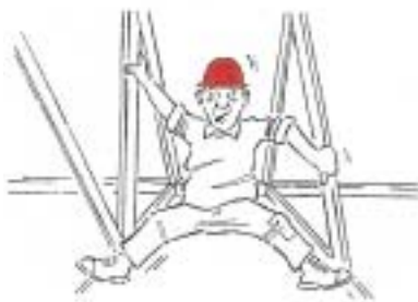
TRUSSES DO NEED BRACING
